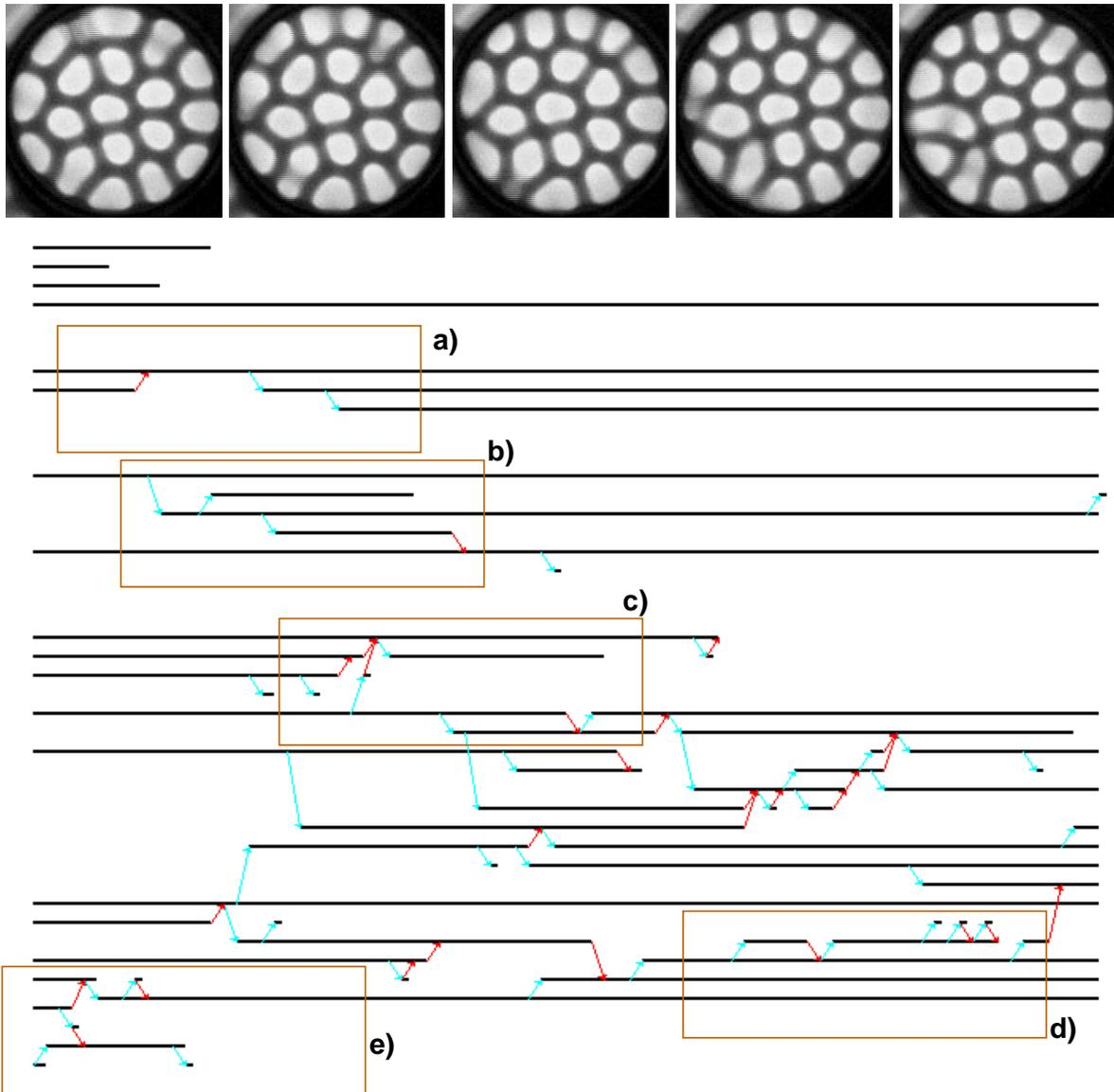
Figure 5: The time-line representation for a combustion experiment exhibiting unstable rings of cells. The images across the top are consecutive frames of videotape of the experiment. Several sections are outlined in the time line for comparison with the corresponding boxes in Figure 6.
