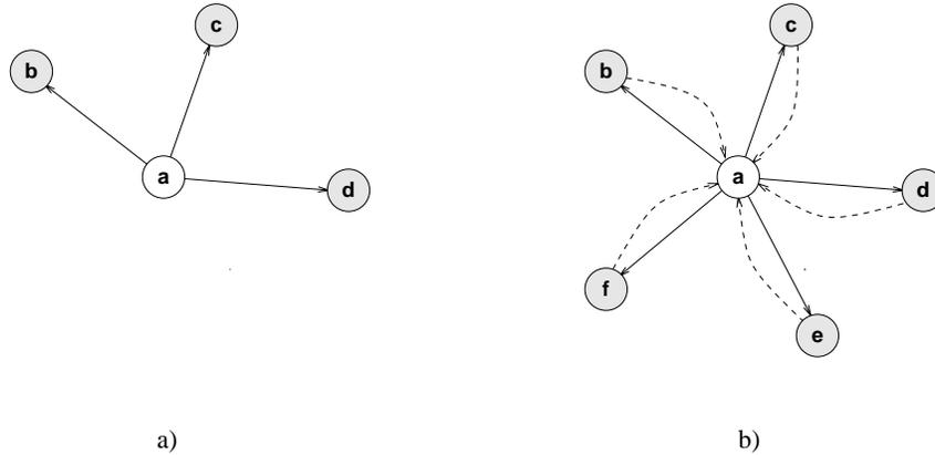
Figure 1: A simple visual model of a broadcast communication with acknowledgments. Node **a** is the sender. The remaining nodes are receivers. a) The state after **b**, **c** and **d** have received the initiation. b) The state after the communication has completed.
