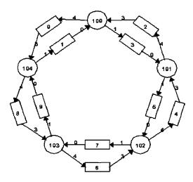
Figure 9: A bidirectional ring of processes.
