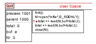
Figure 3: The CPU has been lost during an non-atomic read operation.
