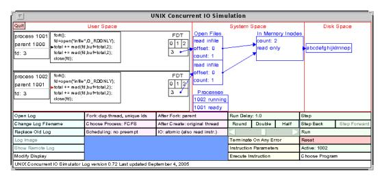
Figure 2: The simulator after a few instruction have been executed.
